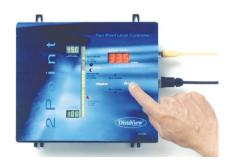
For example, you can use 2Point to control a fill or empty tanks along with a high or low alarm depending on which level is critical to protect. The fill/empty pump range is "latched" internally eliminating additional relays or latching circuits. You can also have an independent high and low control point or even two highs or two low. A DIP switch allows you to configure all these control formats. Three levels of security prevents unauthorized programming changes.
